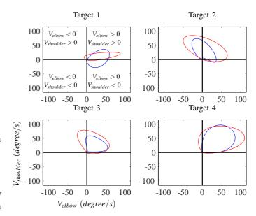
Fig. 8. *PI*<sub>7</sub>: Example of one subject velocity cyclogram during movement to the four targets (Blue: without robot; Red: with robot)
