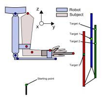
Fig. 3. Schematic of the Codamotion<sup> $\mathbb{R}$ </sup> markers positions during the experiments (In red, markers on the arm, in blue markers on the robot and green markers on the targets)
